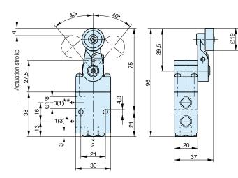
= P when used as "normally closed"= P when used as "normally open" \*\*
