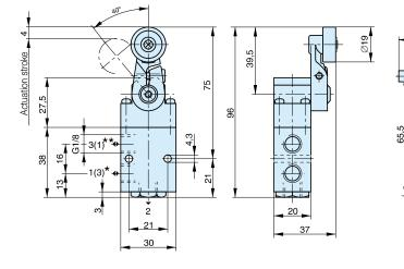
= P when used as "normally closed"= P when used as "normally open" \*;
