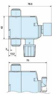
swivel elbow push-in connector 4 mm OD tube
