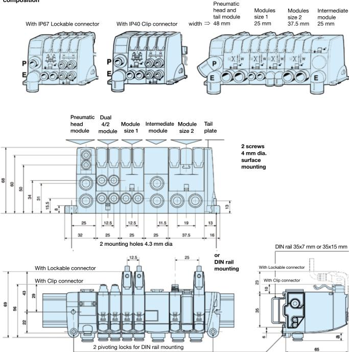
Special case : 4/3 closed centre function within island version : Add the dimensions of the dual P.O. check valve module plugged into the island.
