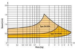
The values relate to an effective driving force of 78 N (6 bar) Shock Absorber Selection in Dependence on Mass and Speed for Series OSP-STL32
