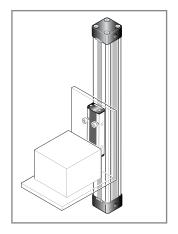
The high load capacity of the piston can cope with high bending moments without additional guides.
