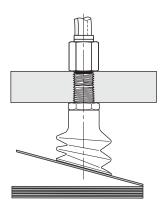
Level compensation for applications where level compensators do not have adequate space
