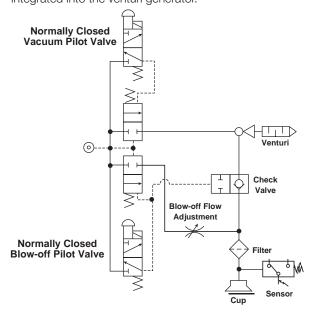
There are several advantages to an integrated venturi system. The response time of the vacuum and blow-off functions are greatly reduced compared to basic venturi generators, the installation time is also reduced which makes this a cost effective system and the compact size allows the integrated unit to be close to the suction cup.
