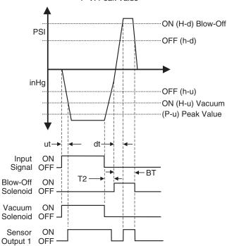
T2: Blow-Off Delay Timer BT: Blow-Off Timer
