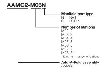
**Example 1:** Application requires an 2-Station MC22 manifold with NPT supply ports.
