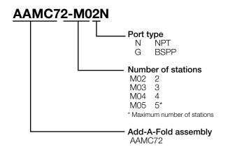
**Example 1:** Shown above is a 2-Station MC72 Manifold with sensors and NPT ports.
