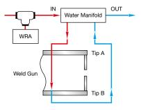
**Scenario 2**, the WRA can be placed on the **OUT** Line of the water manifold. In this situation, you would engage the unit and remove tip A first, replace it, and then remove tip B.
